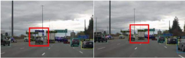
Figure 2: Left: A truck is identified as a van and a car at once. Right: The truck is not detected in the next frame
