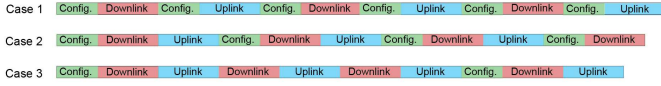
Figure 1: Three TDD cases showing possible allocation of time slots in Individual design (case 1) and joint design (cases 2 and 3). Here, the update overhead and duration are reduced in cases 2 and 3 compared to case 1.
