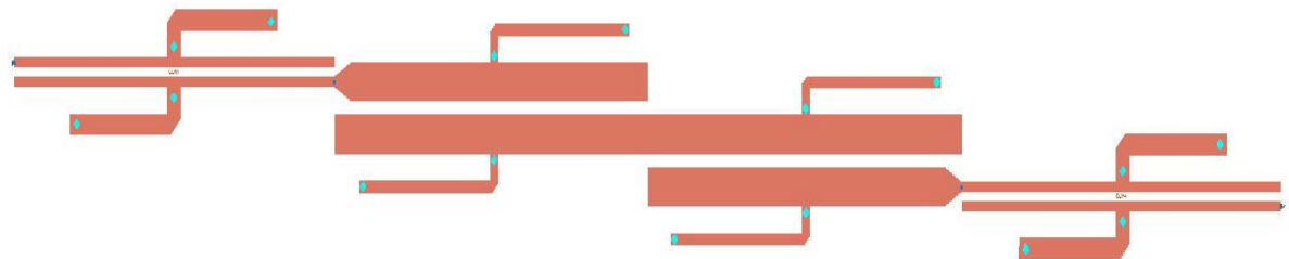
Fig. 6. Coupled line filter with folded T-shaped open-stubs
