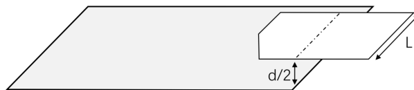
FIG. 5. The system consists of two parallel conducting plates separated by d/2 . The upper plate may have an irregular edge.
