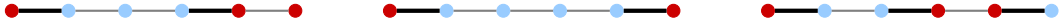
■ Figure 1 The graph P_6 with a matching cut that is not contained in a disconnected perfect matching (left), a matching cut that is properly contained in a disconnected perfect matching (middle) and a perfect matching cut (right). In each figure, thick edges denote matching cut edges.
