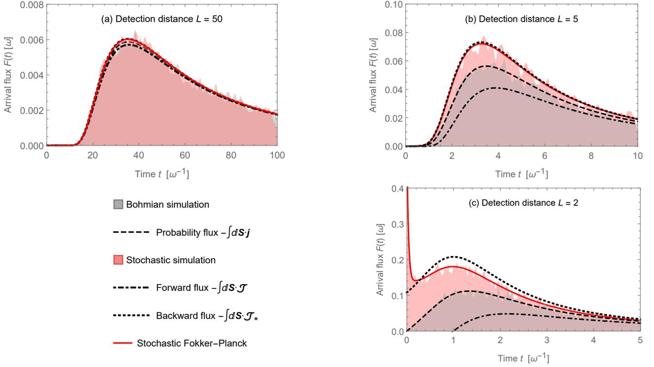
Figure 3: Arrival flux of a cloud of particles released from a single well of frequency  $\omega = \hbar/2m\sigma^2$  and oscillator length  $\sigma$ , onto a detector at different distances  $L$  from the well. (a)  $L = 50\sigma$ ; (b)  $L = 5\sigma$ ; (c)  $L = 2\sigma$ . The Bohmian (grey fill) and stochastic (red fill) arrival fluxes are obtained by sampling 32,000 trajectories propagated from Eqs. (4) and (5) with  $dt = 1/(1600\omega)$ .
