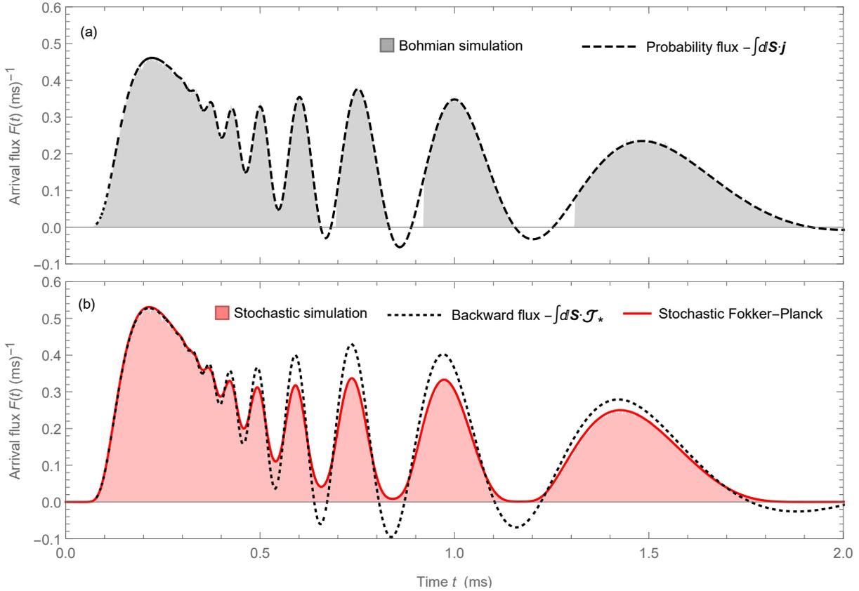
Figure 4: Arrival flux of a cloud of particles released from a double well, onto a detector at a distance  $L = 15\mu\text{m}$  from the centre of the two wells: (a) case of Bohmian trajectories ; (b) case of stochastic trajectories. The fluxes are obtained by sampling  $5 \times 10^6$  trajectories propagated from Eqs. (4) and (5) with  $dt = 3.75 \mu\text{s}$ .
