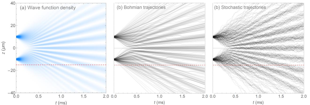
Figure 2: Cloud of particles of mass  $m = 4m_u$  released from two wells of oscillator length  $\sigma = 0.5 \mu\text{m}$ , separated by a distance  $2d = 20 \mu\text{m}$  along the  $z$  direction. The panels are similar to those of Fig. 1. The red dashed line indicates the position of a detector at the distance  $L = 15 \mu\text{m}$  from the centre of the two wells.
