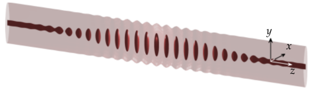
FIG. 1. Example of a stable localized state in a three-dimensional dipolar BEC system. The dipoles are polarized along the y -direction, the BEC is unconfined in the z -direction (axially) and tightly confined in the transverse direction. Even without trap in z -direction, there exist stable localized states which feature a modulated supersolid in the central region and a perfect superfluid sufficiently far from it. This corresponds to an unequal distribution of the local average density. The parameters are n = 5250/\mu\text{m} and a_s = 91a_0 . Contours are given at 1% (light) and 75% (dark) of the peak density. For ease of viewing the z -direction is compressed by a factor 7.
