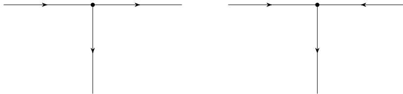
Figure 2: Illustrations of the 1-to-2 T-junction (left), and 2-to-1 T-junction (right).
