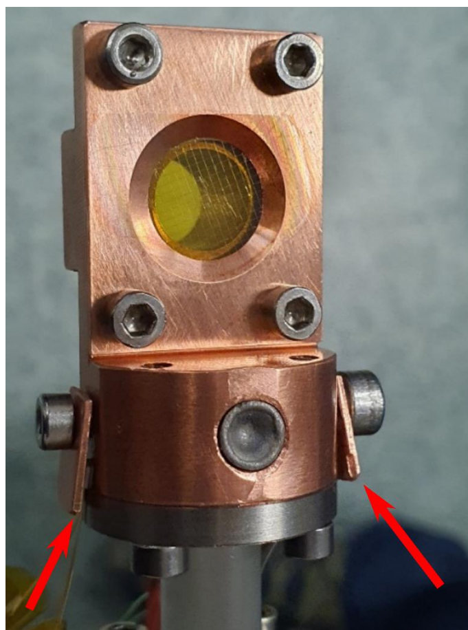
Figure 4. Photograph of the oxygen-free high-conductivity copper sample holder within which a single ZnSe deposition substrate has been mounted. It is possible to note the presence of a thin (<250 nm) gold-wire meshwork on the surface of the ZnSe substrate which serves to preclude the accumulation of electrostatic charge and spark release during ion beam irradiation. Also visible are two of the silicon diodes used to measure the temperature of the sample holder and deposition substrate, indicated by red arrows.
