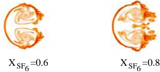
Fig. 3. SF_6 mass fraction at 750\mu s after shock impact. Initial maximum SF_6 mole fraction X_{SF_6}=0.6 on the left, and on the right X_{SF_6}=0.8 .
