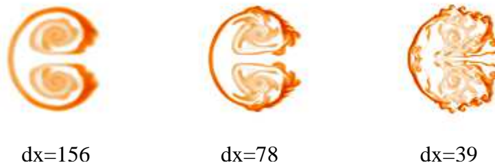
Fig. 4. SF_6 mass fraction at 750\ \mu s with increasing grid resolution, labeled in microns. At the highest level of resolution, the vortex cores appear diffuse.
