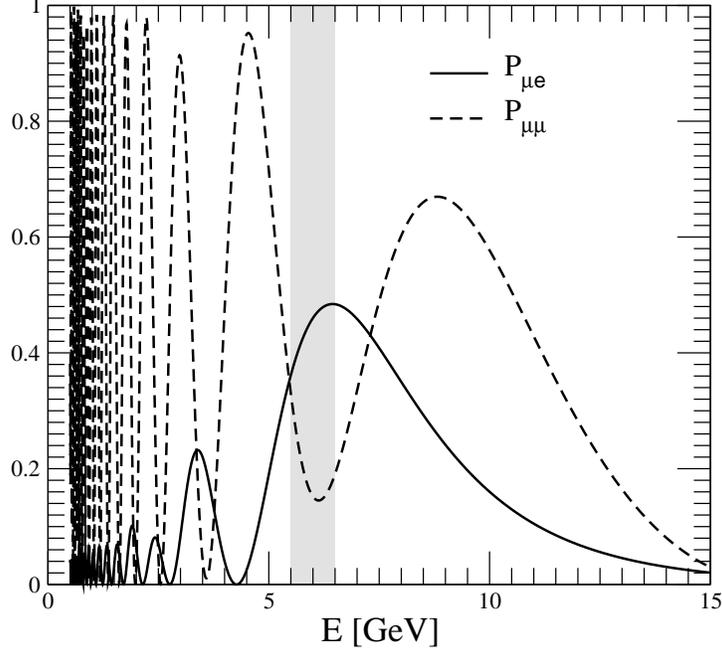
FIG. 2: The transition probabilities  $P_{\mu e}$  and  $P_{\mu\mu}$  for a baseline length  $L = 9300$  km with  $\sin^2 2\theta_{13} = 0.1$ ,  $\sin^2 2\theta_{23} = 1$  and  $\delta_{cp} = 0$ . The gray zone represents the region with the neutrino energy  $E_\nu$  ranging from 5.5 GeV to 6.5 GeV, where the maximum of  $P_{\mu e}$  and the local minimum of  $P_{\mu\mu}$  are located.
