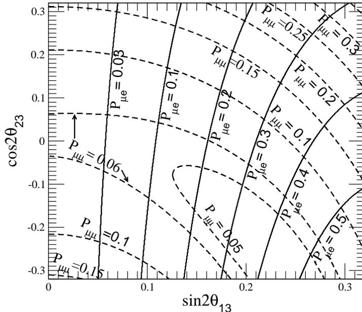
FIG. 3: The contour graph of the transition probabilities  $P_{\mu e}$  (solid line) and  $P_{\mu\mu}$  (dashed line) in the  $\sin 2\theta_{13}$ - $\cos 2\theta_{23}$  plane for  $\delta_{CP} = 0$  and the baseline length  $L = 9300$  km. The plotted  $P_{\mu e}$  and  $P_{\mu\mu}$  are the averaged probabilities for neutrino energies ranging from 5.5 GeV to 6.5 GeV
