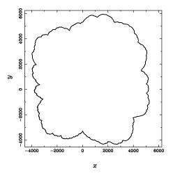
FIG. 1. Simulations of the outward propagating flame front. Note that there is a wide distribution of cusp sizes.
