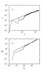
FIG. 2. Panel a: a logarithmic plot of the velocity versus time for a radially evolving system. The parameters of the simulation are:  $f = 10^{-8}$ ,  $\gamma = 0.8$ ,  $\nu = 1$ . Panel b:Logarithmic plot of the width of the flame front as a function of the mean radius.
