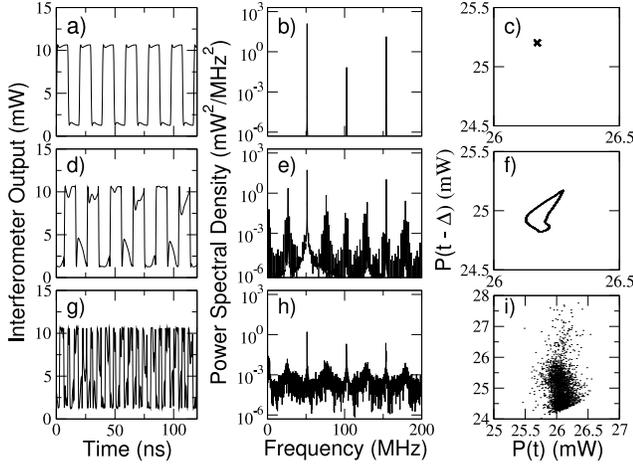
Fig. 6. Numerical time series (panels a,d,g), power spectra (panels b,e,h), and Poincaré sections (panels c,f,i) are shown. The gain values are as in Fig. 5, that is,  $\gamma = 9.4$  mV/mW (a,b,c),  $\gamma = 13.2$  mV/mW (d,e,f), and  $\gamma = 17.6$  mV/mW (g,h,i).
