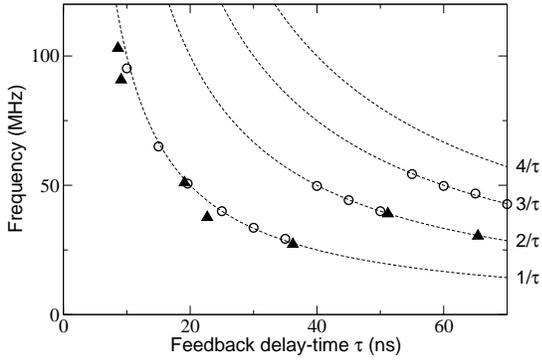
Fig. 4. Frequency of the oscillations close to the Andronov-Hopf bifurcation point versus the feedback delay time  $\tau$ . Measured (triangles) and numerically estimated (circles) frequencies are shown. We display curves  $n/\tau$  with  $n = 1, 2, 3, 4$  for visual guidance.
