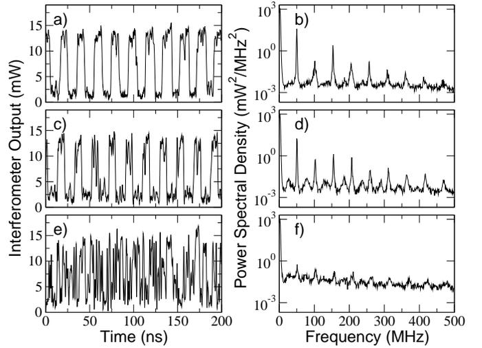
Fig. 5. Experimentally measured time series (panels a,c,e) and power spectra (panels b,d,f) obtained from the second output port of the interferometer are shown.  $\gamma = 9.4$  mV/mW for a) and b),  $\gamma = 13.2$  mV/mW for c) and d), and  $\gamma = 17.6$  mV/mW for e) and f).
